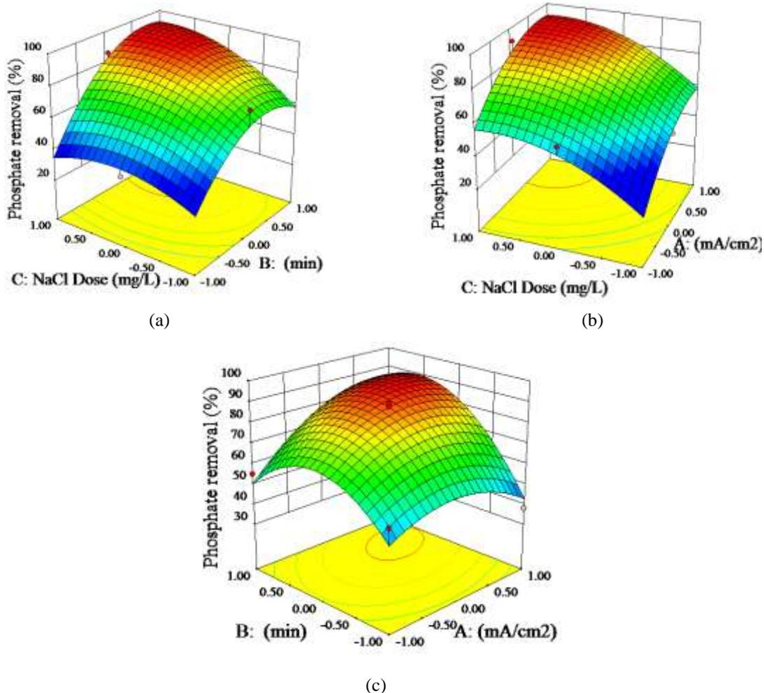
Fig. 03 Contour plots for % phosphate removal as a function of (a) NaCl dose and time (b) current density NaCl dose (c) time and current density
